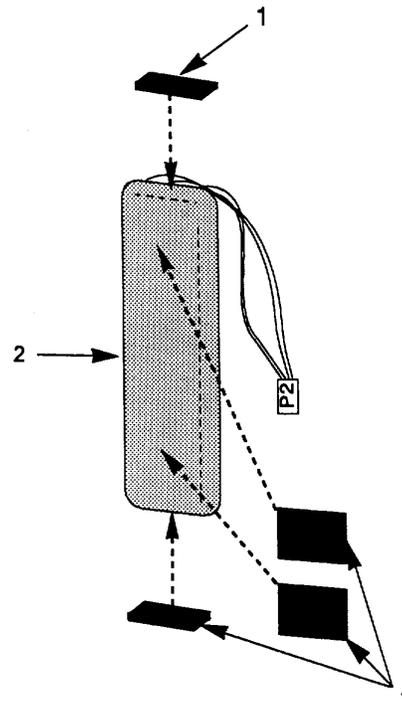
(2) Place the battery pack (2) in the bracket assembly (1) by pivoting the battery pack at a 45-degree angle and sliding into place.
