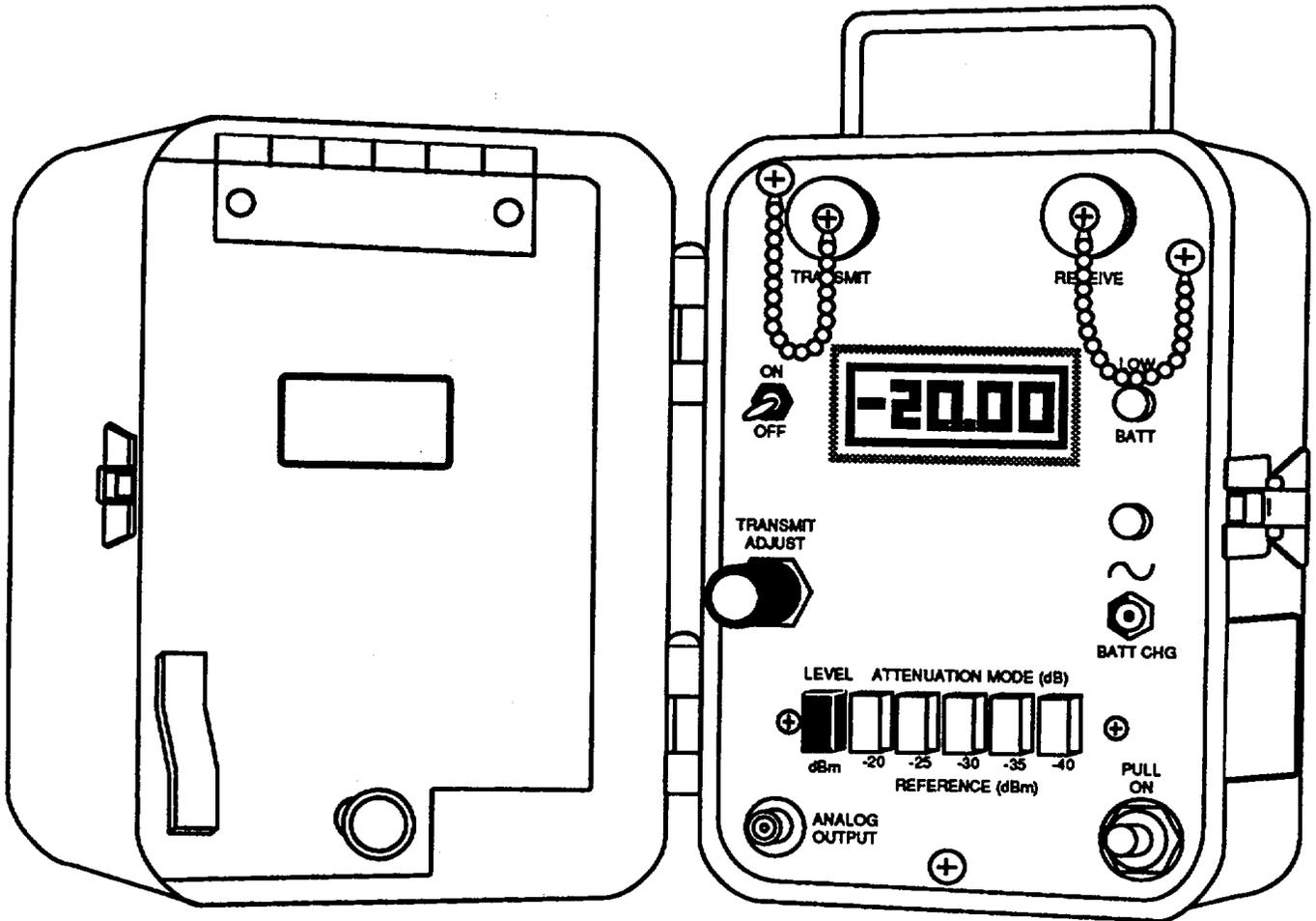
Figure 1-1. Optical Fiber Test Set TS-4335/G
