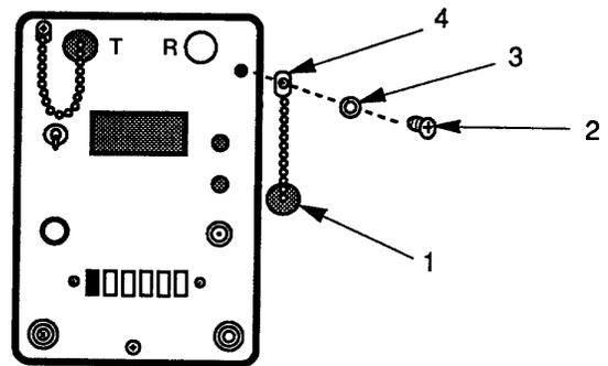
**b. LEVEL/ATTENUATION MODE Pushbutton Replacement.** Replace the LEVEL and ATTENUATION MODE pushbuttons as follows:
